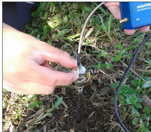
Figure 6. Measuring antenna resistance
