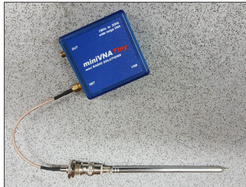
Figure 2. Telescopic VHF radio antenna attached to the miniVNA Tiny
